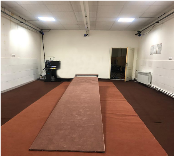
Figure 2: Walkway constructed with the slope of 8°
