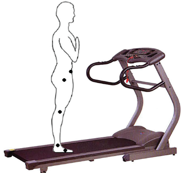
Figure 2: The schematic diagram of reflective markers attached to the skin
