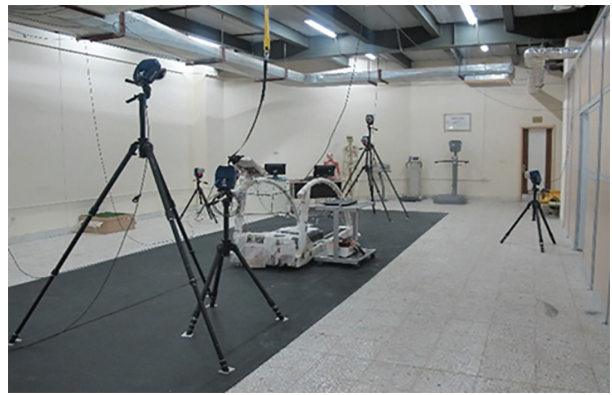
Figure 1: 3D analyzer with 6 infrared optoelectronic cameras
