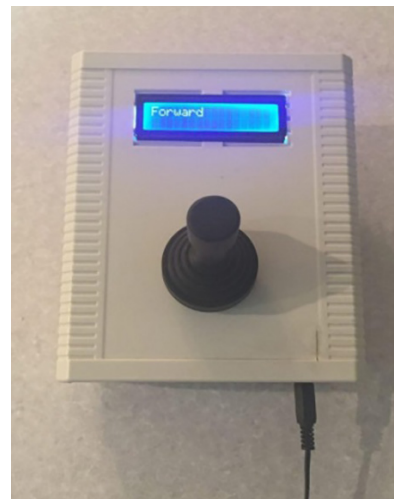
Figure 6: The joystick handle designed to control the movement of the orthosis (installed on control unit box)
