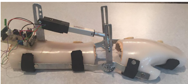
Figure 10: The protpotype of active wrist orthosis
