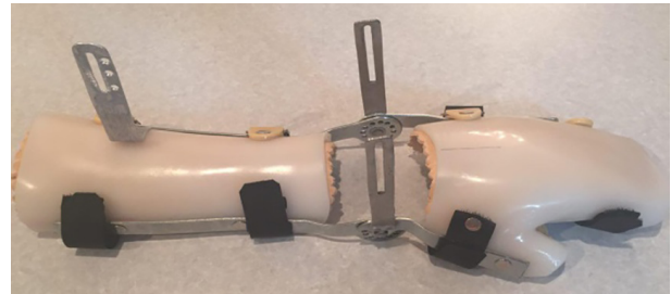
Figure 5: The main body of wrist orthosis with linkages and retaining straps
