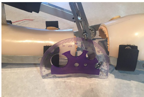
Figure 13: The measurement of the maximum orthosis rotation angle in the direction of wrist extension
