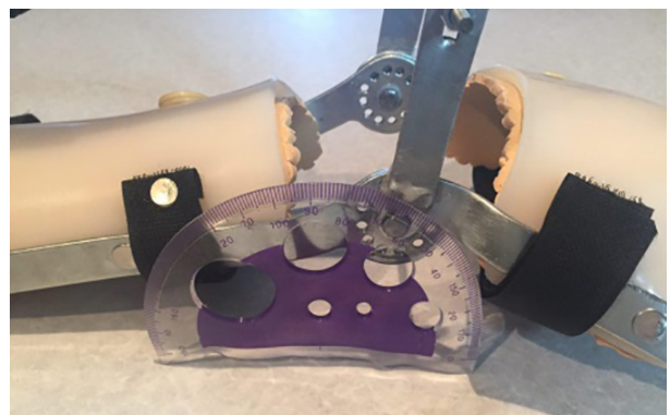
Figure 12: The measurement of the maximum orthosis rotation angle in the direction of wrist flexion
