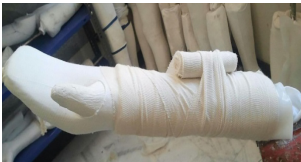
Figure 4: The prepared mold to form the thermoplastic sheet
