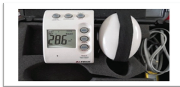
Figure 1: Handheld digital dynamometer
