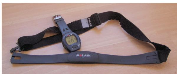
**Figure 2:** Polar heart rate monitoring system
